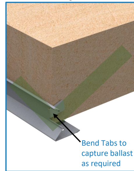
Bend tabs at ends of Ballast Rail (See 5.2 to determine if required)
